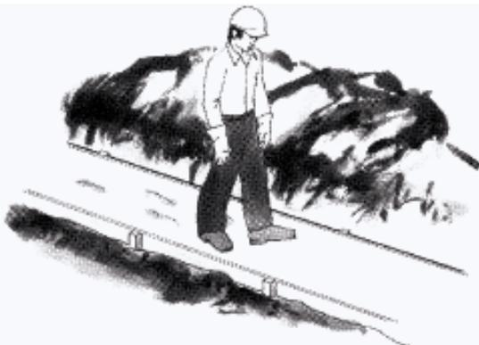
8. Walk on consolidated **GILSULATE® 500XR** envelope to ensure use density, footprints less than 1" deep are required.
